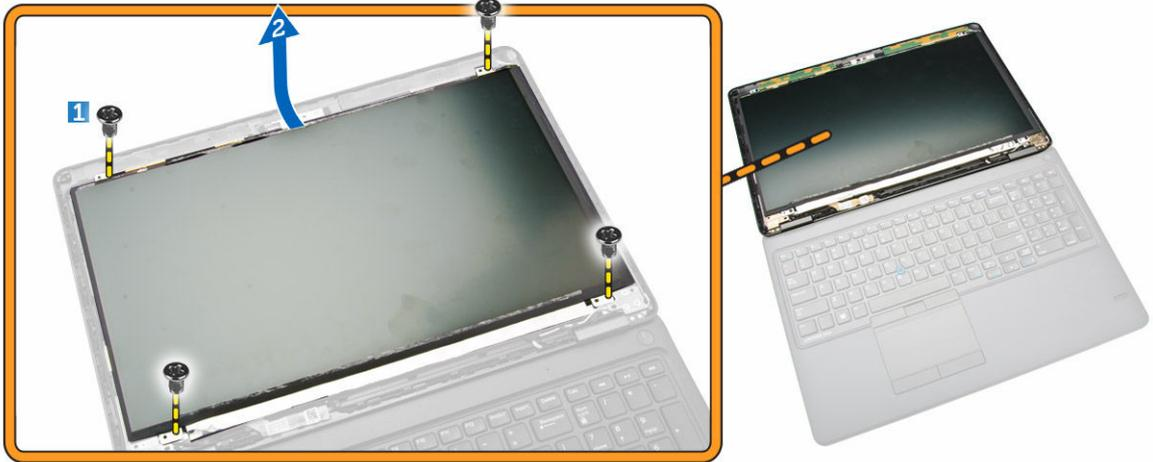
4. Peel the adhesive [1] to access the eDP cable [2].
