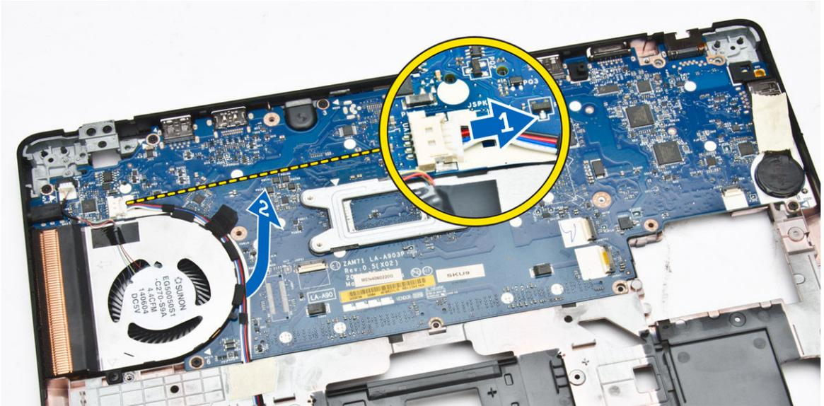
4. Remove the screws that secure the system board to the chassis.
