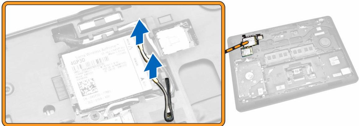
4. Remove the screw that secures the WWAN card [1] and remove the WWAN card from the computer [2].
