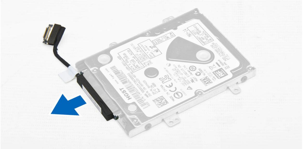
6. Remove the screws that secure the hard-drive bracket to the hard drive [1] and remove the hard drive from the hard-drive bracket [2].
