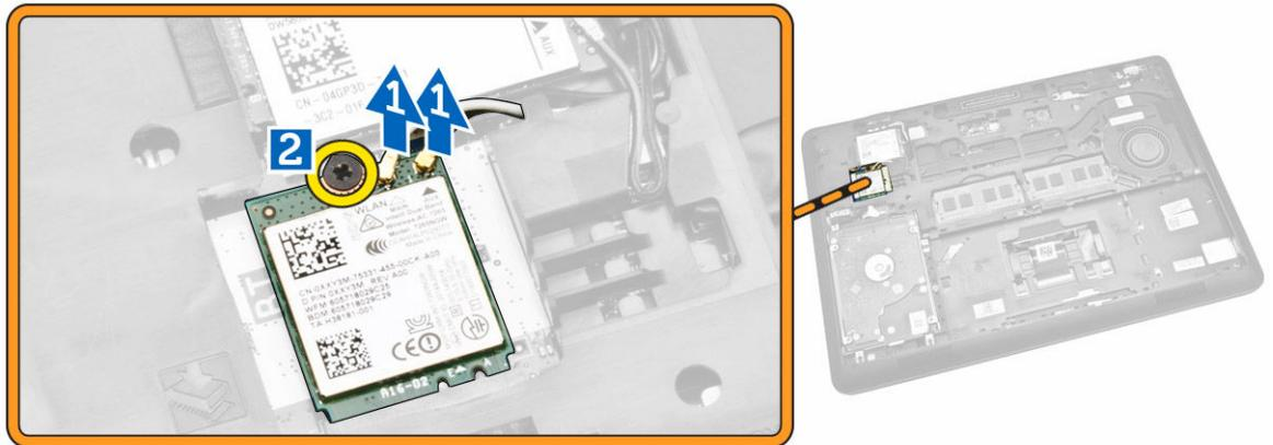
4. Remove the WLAN card from the computer.
