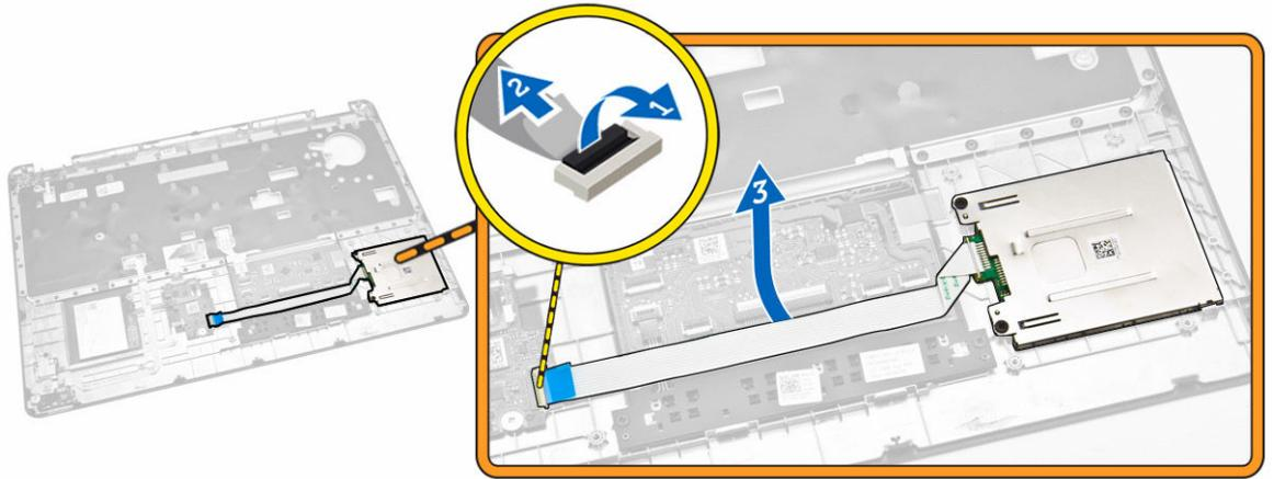
4. Release the SmartCard reader board. To release the SmartCard reader board:
