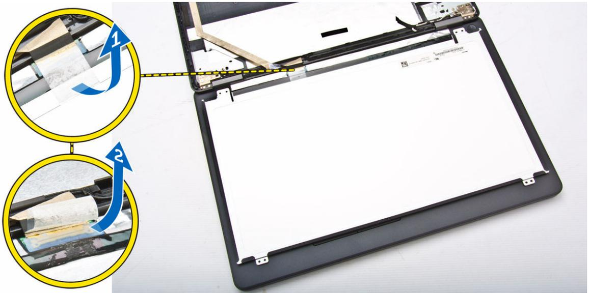
5. Disconnect the eDP cable from its connector [1] and remove the display panel from the display assembly [2].
