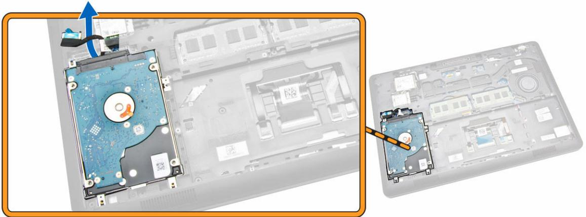
5. Pull to release the hard-drive cable from its connector.
