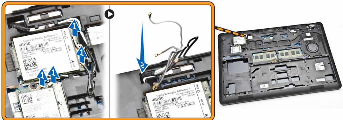
4. Perform the following steps to disconnect the display cable from the system board:
